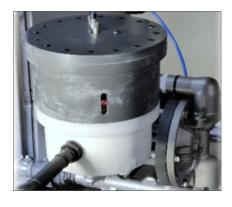
If installation space is limited, the Inline Dampener can be mounted in each position directly on the pump.
